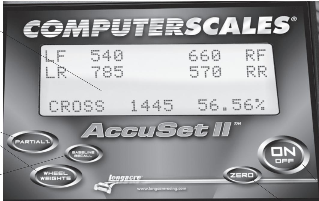
Display shuts off after 90 minutes. If needed simply turn back on. No need to remove car or re-zero.
