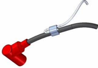
Wrapping of RPM cable on spark cable
