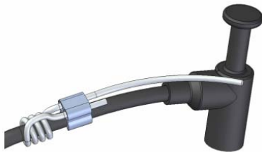
Wrapping of RPM cable on spark cable
