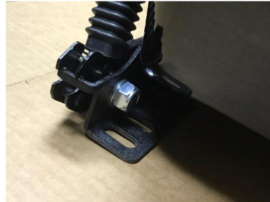
Step 3. Attach side mounts to aftermarket seats, using the hardware included with the seats. It is recommended that you fully tighten the inside (center console side) seat mount to mount bolts, but leave the outside seat mount somewhat loose until installed in the car. Seat height is set by the rear hole, seat tilt is set by the front holes.
